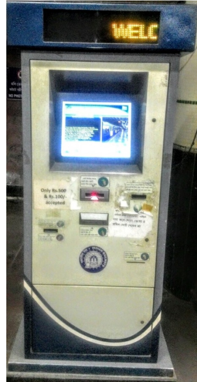
ASCRM being used by Kolkata Metro at stations for purchasing new Smart Card and recharging existing Smart Card
