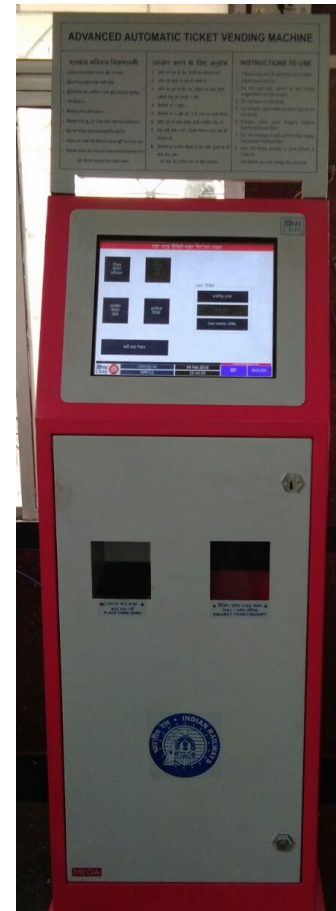
Image of ATVM machine being used by Indian Railways at stations for issuing Unreserved Tickets.
